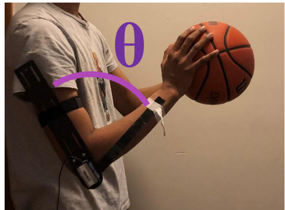
Figure 4: The Experimental Setup, Diagram of Sensors with respect to the player. Goniometer strapped to player's arm. Designated Starting Position of each shot (i.e Minimum Angle). Measured angle theta shown in purple.
