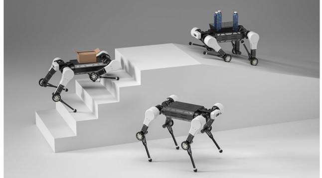
Fig. 1. Multiple quadruped robots performing collaborative lifting tasks. The versatility of legged platforms is showcased by their ability to adjust step size and climb elevated terrain efficiently; making them ideal for applications like search and rescue and urban locomotion.
